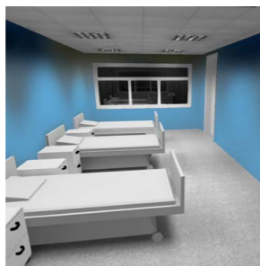
The classical lighting solution in bedrooms with recessed luminaires with a parabolic louvre ensures sufficient illumination of the rooms but the upper parts of the walls and the ceiling remain dark. Such illumination causes a feeling of a cave effect and makes the room optically smaller.
