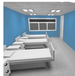
The sufficient illumination of the ceiling can be achieved by using the luminaire with the direct luminous flux distribution combined with the illumination of the ceiling thanks to the specially shaped diffuser. The room then gives an impression of a lighter and larger space.
