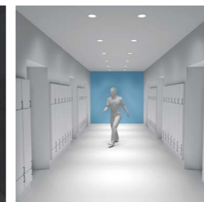
When someone enters the room, the presence detector responds to the infrared radiation the human body emits and switches on the lighting.
