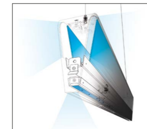
An interesting luminaire design in terms of its ability directs the light in a biologically effective way. The direct light directed from the LED sources located in the bottom part of the construction is completed by a microprismatic diffusor that alters the direct light into soft, diffused light. The side optics are designed in such a way
