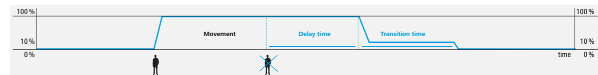
When someone enters the room, the presence detector responds to the infrared radiation the human body emits and switches on the lighting.
